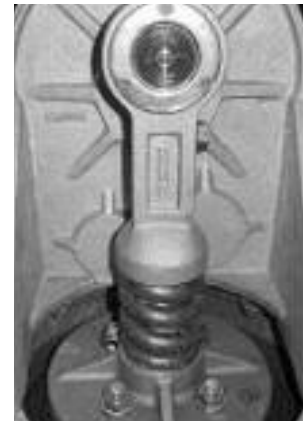
Spring loaded connecting rod. Prevents damage to water box and transmission from solids and sediment.
